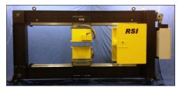
The GaugeMaster system is a high performance coating weight gauge featuring low noise and fast response for the most demanding applications. High power x-ray sources are employed to provide better noise-to-signal ratios for
