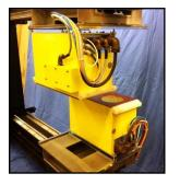
improved control, product quality and productivity. Differential ion chambers with selected filters ensure high sensitivity and immunity from Compton backscatter effects.
